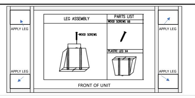
The plastic legs should be evenly aligned on each corner of the unit, approximately 1/4" - 3/8 " from each edge. Place 2 screws, one in each of the screw hole. Secure the legs to the frame using a hex-head screwdriver bit and a power drill.
