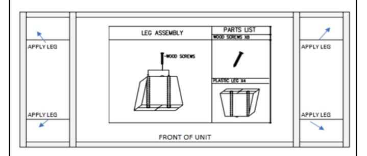
The legs should be evenly aligned on each bottom corner of the unit, approximately 1/4" - 3/8 " from the edge. Place 2 screws, one in each of the screw holes. Secure the legs to the frame using a hex-head screwdriver bit and a power drill. **Do not over tighten screws.**
