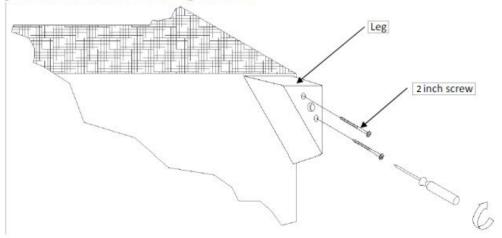
Repeat steps 1 and 2 for the remaining legs. Turn the unit upright and place in the desired location.
