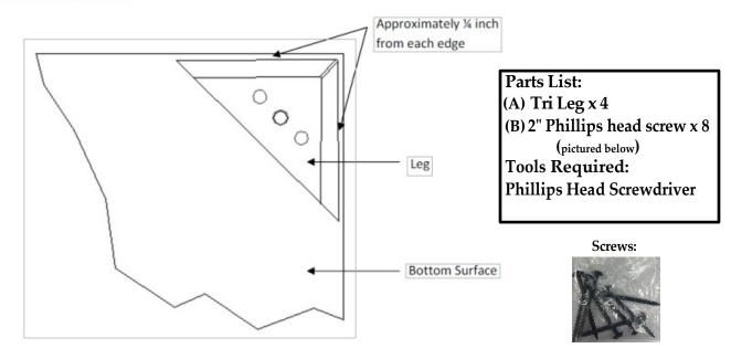
Step 2 – Fasten the leg by inserting (2) - 2 inch screws per leg in the holes provided and screw until the leg is secure.
