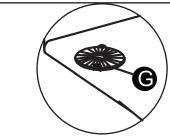
Adjust each leg by inserting a washer (G) to make it even and level with the floor.
