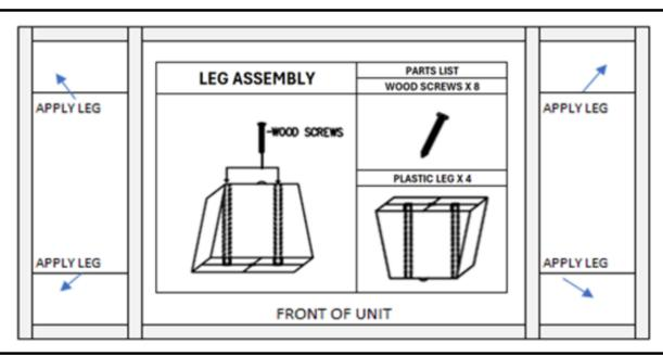
The legs should be evenly aligned on each bottom corner of the unit, approximately 1/4" - 3/8 " from the edge. Place 2 screws, one in each of the screw holes. Secure the legs to the frame using a hex-head screwdriver bit and a power drill. **Do not over tighten screws.**
