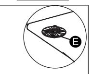
Adjust each leg by inserting a washer E) to make it even and level with the floor.
