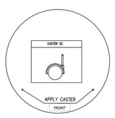
Locate the 2 metal inserts on the bottom, front surface of the chair. Using hand pressure only, slide the metal stem of the caster into the metal inserts, until the casters snap in place. **Do not** use a hammer or other object to force the casters, as this will result in damage.
