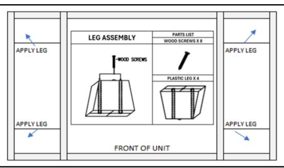
The legs should be evenly aligned on each bottom corner of the unit, approximately 1/4" - 3/8 " from the edge. Place 2 screws, one in each of the screw holes. Secure the legs to the frame using a hex-head screwdriver bit and a power drill. **Do not over tighten screws.**
