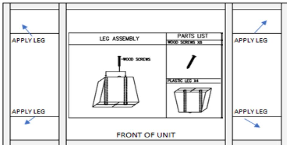
The legs should be evenly aligned on each bottom corner of the unit, approximately 1/4" - 3/8 " from the edge. Place 2 screws, one in each of the screw holes. Secure the legs to the frame using a hex-head screwdriver bit and a power drill. **Do not over tighten screws.**
