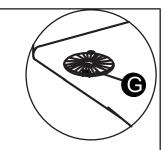
Adjust each leg by inserting a washer (G) to make it even and level with the floor.
