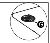
Adjust each leg by inserting a washer (G) to make it even and level with the floor.
