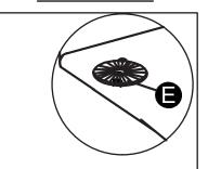
Adjust each leg by inserting a washer E) to make it even and level with the floor.
