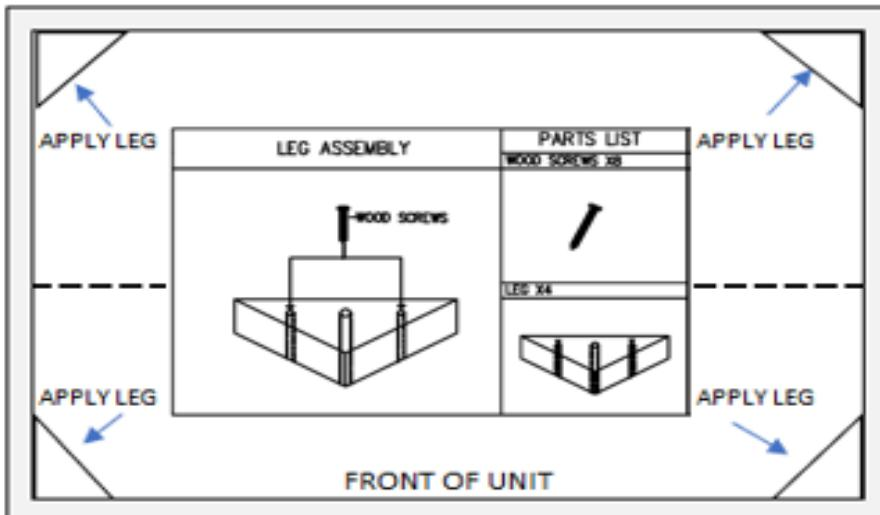
The triangle legs should be evenly aligned on each bottom corner of the unit, approximately 1/4" - 3/8" from the edges. Place 2 screws, one in each of the screw holes. Secure the legs to the frame using a hex-head screwdriver bit and a power drill. **Do not over tighten screws.**
