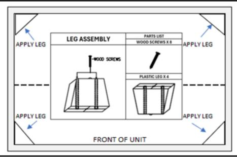
The legs should be evenly aligned on each bottom corner of the unit, approximately 1/4" - 3/8" from the edges. Place 2 screws, one in each of the screw holes. Secure the legs to the frame using a hex-head screwdriver bit and a power drill. **Do not over tighten screws.**
