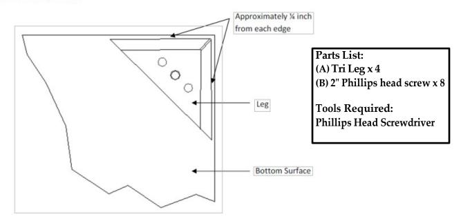
Step 2 – Fasten the leg by inserting (2) - 2 inch screws per leg in the holes provided and screw until the leg is secure.
