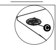
Adjust each leg by inserting a washer (C) to make it even and level with the floor.
