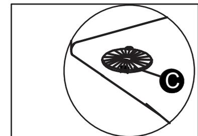
Adjust each leg by inserting a washer (C) to make it even and level with the floor.
