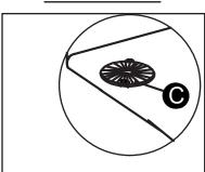
Adjust each leg by inserting a washer (C) to make it even and level with the floor.
