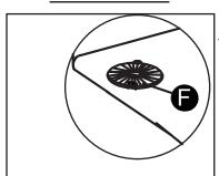
Adjust each leg by inserting a washer (F) to make it even and level with the floor.
