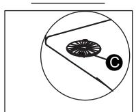
Adjust each leg by inserting a washer (C) to make it even and level with the floor.
