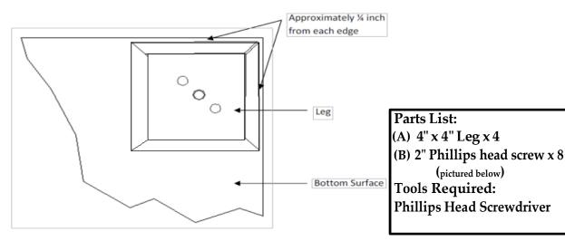
Step 2 – Fasten the leg by inserting (2) – 3 inch screws per leg in the holes provided and screw until the leg is secure.
