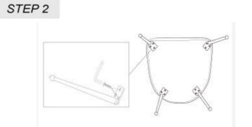
> Please find the hole which marked at bottom. Put legs at the right location.> Fix the screws by wrench on the hole one by one. Total 3 screws for one leg.> Fix other legs as the same way as first one
