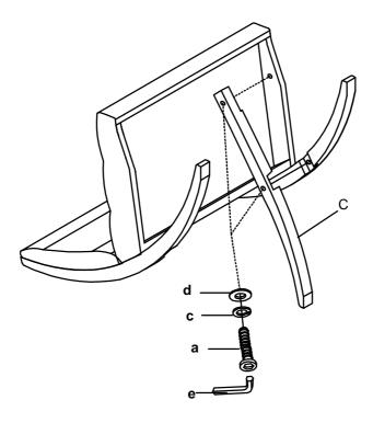
Step 3: Repeat the Step to assemble the other front leg (D). Securely tighten all bolts by Allen wrench (e), but do not over tighten the bolts. Assembly is complete.
