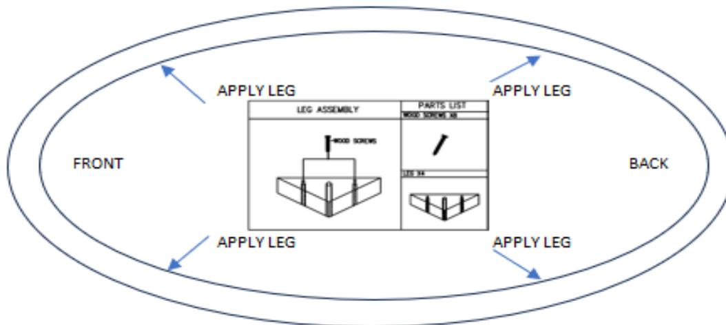
The legs should be evenly aligned on each side of the unit, approximately 1/4" - 3/8" from the edge. Place 2 screws, one in each of the screw holes. Secure the legs to the frame using a hex-head screwdriver bit and a power drill. **Do not over tighten screws.**
