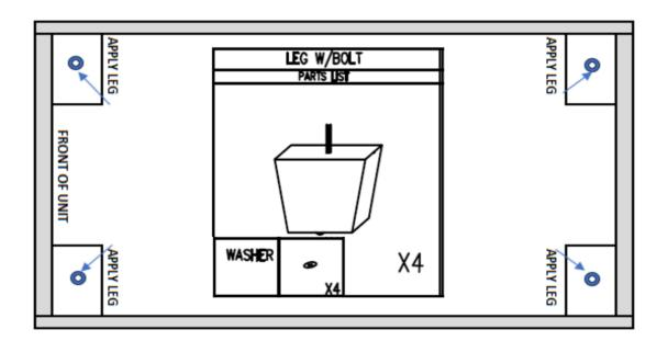
Align the hanger bolt with the threaded insert, on each bottom corner of the unit. Insert the bolt and turn the leg clockwise, until fully seated.
