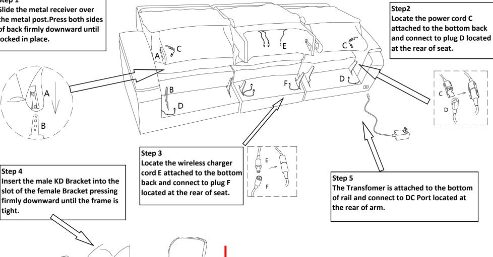
Note: Make sure all PLUGS are connected on the product before plugging power cord into power outlet. If not damage can occur. The USB ports (where applicable) are designed with working voltage of 5V, and can NOT be used to supply power for laptop computers (neither PC or Mac). Plugging a laptop computer to the USB port may end up damaging either the computer or the USB port due to unmatched working voltage.
