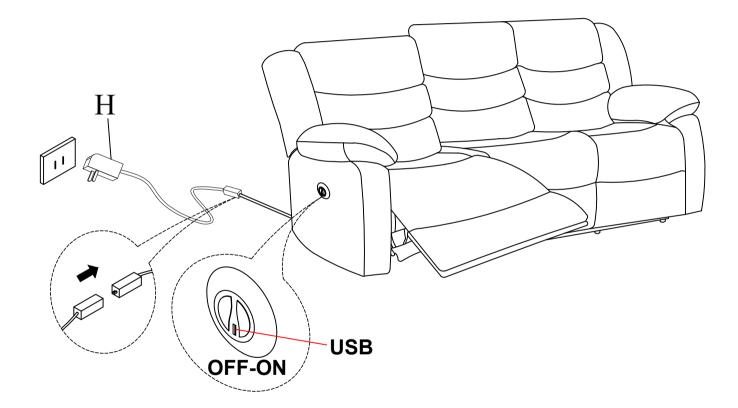
Connect the power and Open the footrest by pressing the button.
