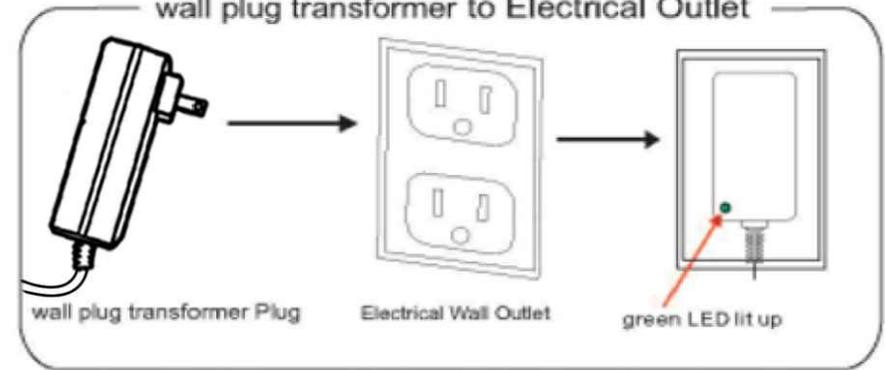
After all connections have been made,ensure that the LED light is lit on after the transformer is power on.
