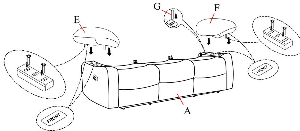
**Attach the Left/Right Armrest (E/F) to the Seat (A) by using the Fixed latch (G).**
