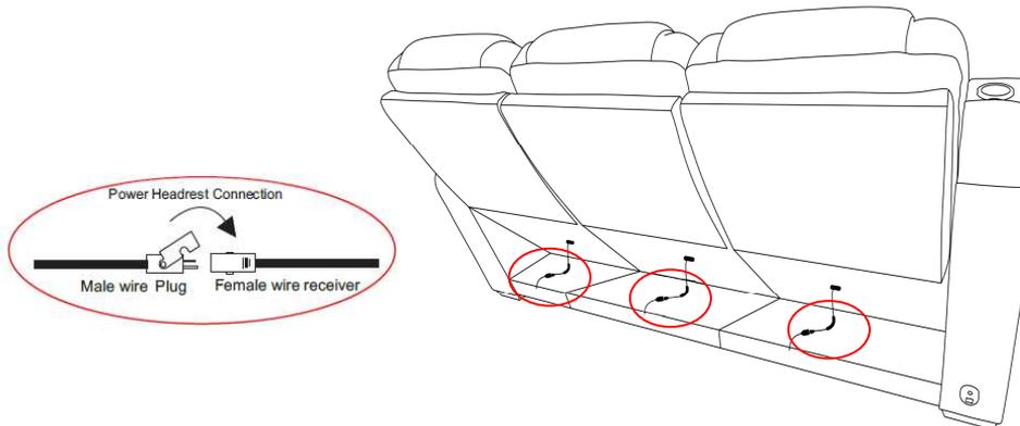
**Step 4:** Latch male wire plugs from middle backrest to female wire receivers located at the bottom back underneath the flap. Connecting for reading lights & wireless charger.
