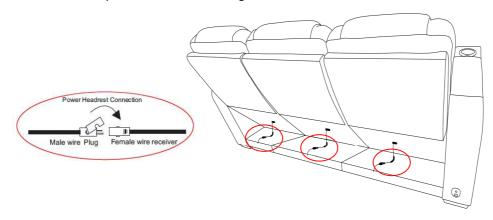
**Step 4:** Latch male wire plugs from middle backrest to female wire receivers located at the bottom back underneath the flap. Connecting for reading lights & wireless charger.
