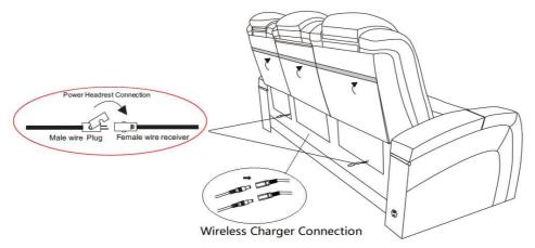
**Step 4:** Latch male wire plugs from middle backrest (wireless charger) to female wire receivers located at the bottom back underneath the flap.
