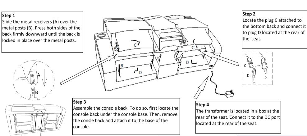
Note: Make sure all plugs are connected on the product before plugging power cord into power outlet. If not, damage can occur. The USB ports (where applicable) are designed with working voltage of 5V, and can NOT be used to supply power for laptop computers (neither PC or Mac). Plugging a laptop computer to the USB port may end up damaging either the computer or the USB port due to unmatched working voltage.
