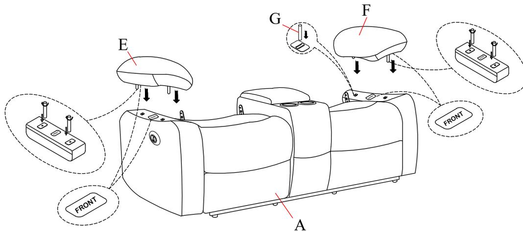
**Attach the Left/Right Armrest (E/F) to the Seat (A) by using the Fixed latch (G).**
