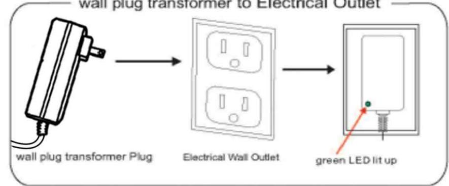
After all connections have been made, ensure that the LED light is lit on after the transformer is power on.
