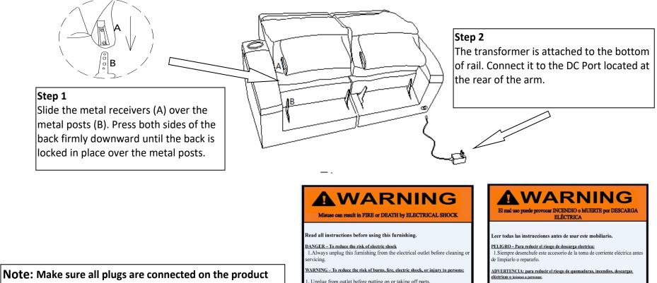
before plugging power cord into power outlet. If not, damage can occur. The USB ports (where applicable) are designed with working voltage of 5V, and can NOT be used to supply power for laptop computers (neither PC or Mac). Plugging a laptop computer to the USB port may end up damaging either the computer or the USB port due to unmatched working voltage.
