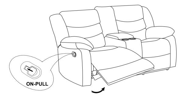
Open the Footrest by pulling out the Switch
