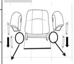
LINE-UP THE MALE AND FEMALE BRACKETS AND ASSEMBLE THE K/D WINGS ON 2 SIDES OF SOFA BACK.
