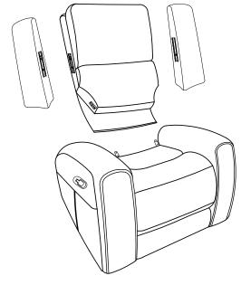
Take out the KD(C&D) wings underneath the Laf and Raf a rms which fixed by the ropes, then you can remove the ropes away.
