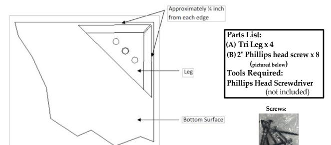
Step 2 – Fasten the leg by inserting (2) – 2 inch screws per leg in the holes provided and screw until the leg is secure.
