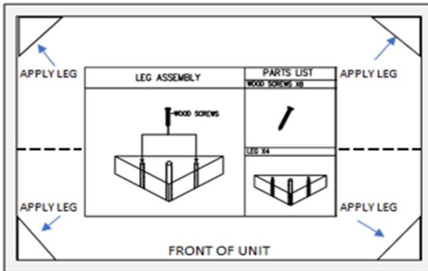
The legs should be evenly aligned on each bottom corner of the unit, approximately 1/4" - 3/8" from the edge. Place 2 screws, one in each of the screw holes. Secure the legs to the frame using a hex-head screwdriver bit and a power drill. **Do not over tighten screws.**
