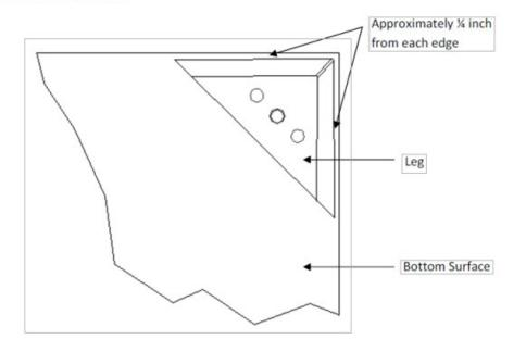
Step 2 – Fasten the leg by inserting (2) - 2 inch screws per leg in the holes provided and screw until the leg is secure.
