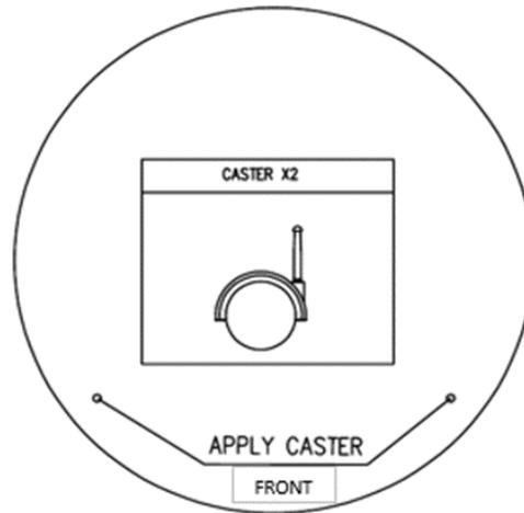
Locate the 2 metal inserts on the bottom, front surface of the chair. Using hand pressure only, slide the metal stem of the caster into the metal inserts, until the casters snap in place. **Do not** use a hammer or other object to force the casters, as this will result in damage.
