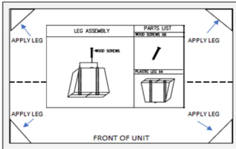
The legs should be evenly aligned on each bottom corner of the unit, approximately 1/4" - 3/8" from the edges. Place 2 screws, one in each of the screw holes. Secure the legs to the frame using a hex-head screwdriver bit and a power drill. **Do not over tighten screws.**
