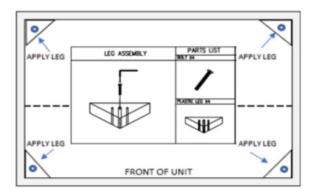
The legs should be evenly aligned on each bottom corner of the unit. Place and allen bolt in the center hole of the leg and align with the threaded insert. Using the wrench, turn the bolt clockwise, until fully seated.
