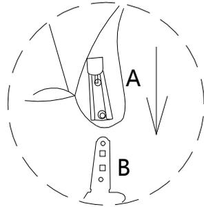
1、 Slide the metal receiver over the metal post. Press both sides of back firmly downward until locked in place.
