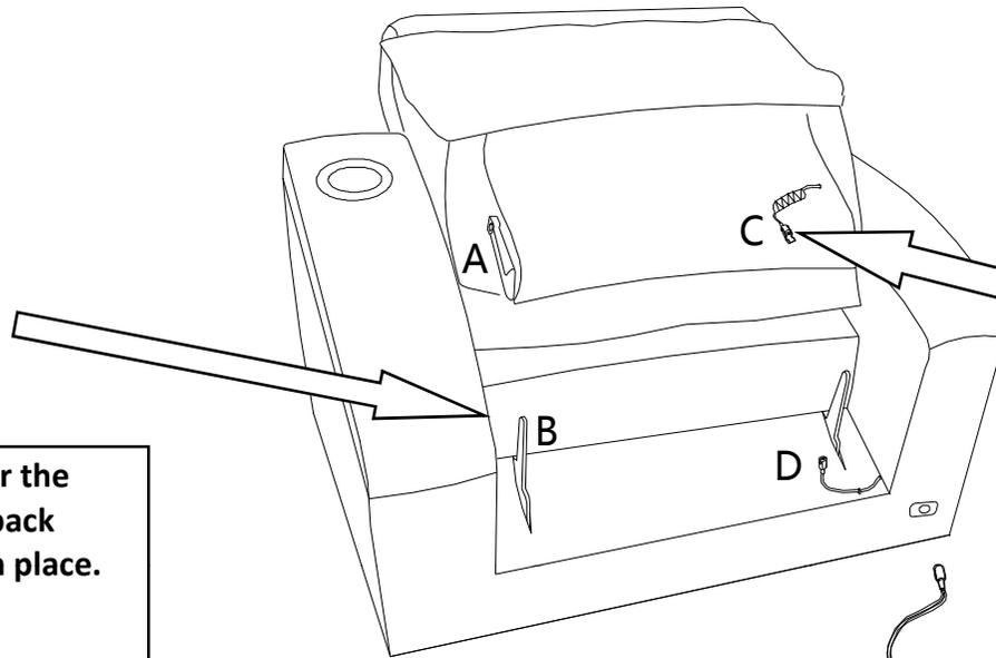
2、 Locate the power cord C attached to the bottom back and connect to plug D located at the rear of seat.
