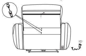
**STEP 1: Attach the KD back(s)** Check to assure both sides of the mechanism post are positioned inside of the KD receivers on the sides of the back frame, push in a downward motion from the top of the back frame until a clicking sound is heard.
