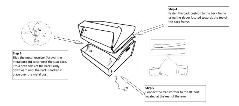
**Note:** Make sure all plugs and cords are connected on the product before plugging the power cord into power outlet. Otherwise, damage can occur.
