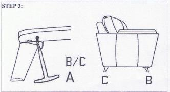
Please screw the bolts clockwise on the 4 side feet into the plate, until fully in position.
