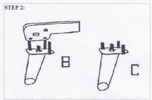
Install the high bolts into the short leg and the short bolt into the high leg.
