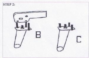
Install the high bolts into the short leg and the short bolts into the high leg.
