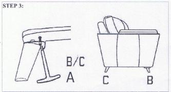
Please screw the bolts clockwise on the feet into the plate, until fully in position.
