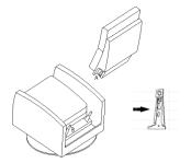
**2**. Press both sides of the back firmly downward until the back is locked in place over the metal post.
