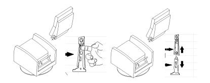
**3**. To remove the back from the seat, lift the tab on both sides and pull the back straight up until it is free from the seat.
