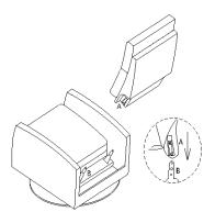
**1**. Slide the metal receiver (A) over the metal post (B) to connect the seat back.
