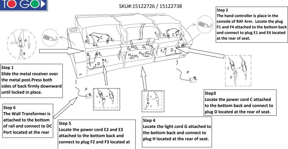
**Note:** Make sure all PLUGS are connected on the product before plugging power cord into power outlet. If not damage can occur.
